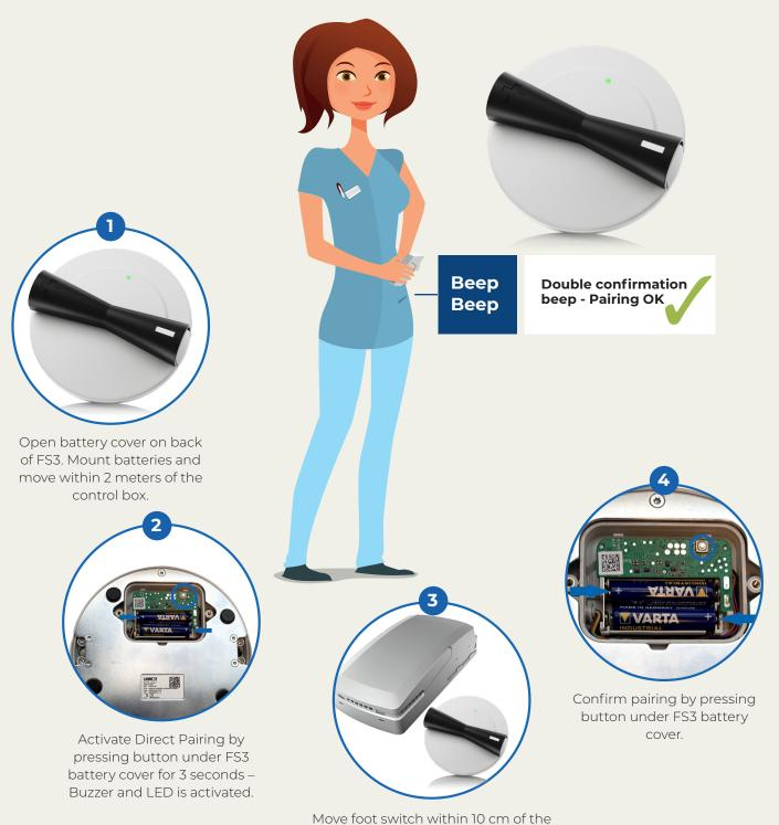
control box until buzzer frequency change from slow to fast.
