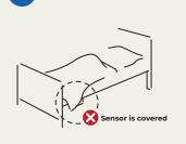
The sensor field of vision is obstructed, in this case by the bed sheets and will not function. Bed light with motion sensor
