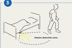
Patient walks away from the bed and exits the motion detection zone. After 10 seconds of inactivity the guiding light dim down.
