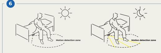
The guiding light will only turn on in poorly lit rooms. (Guiding light will turn on when night threshold is below approximately 35 lux. Guiding light will not turn on when light is above approximately 75 lux
