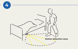
Patient returns to the bed, activates the bed sensor and guiding light is back on max intensity. When the patient enters the bed again, the guiding light will dim down after 10 seconds and turn off after 10 minutes.
