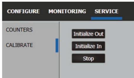
From here, determine where your actuator's current position is. If the actuator is fully extended, then select "Initialize In" to run the actuator to the inwards limit switch. If the actuator is fully retracted, then select "Initialize Out" to run the actuator to the outwards limit switch. If the actuator is somewhere in between fully extended and fully retracted, selecting either "Initialize In" or "Initialize Out" will successfully calibrate the system.
