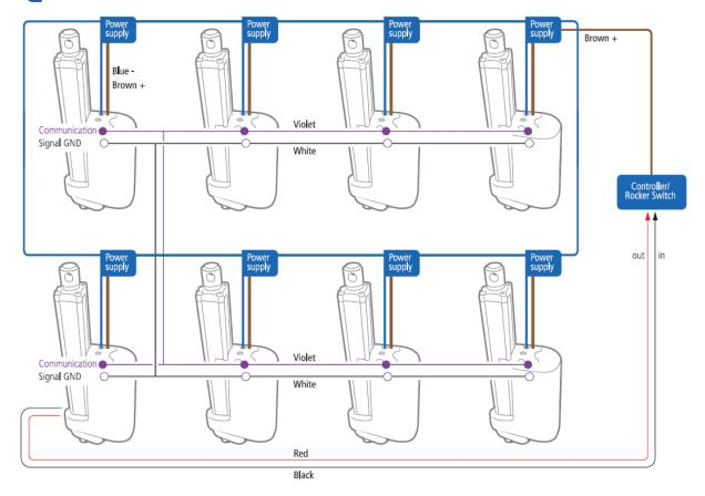
Only standard power and signal cables are available for parallel.
