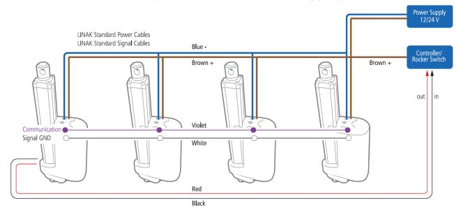
It is both possible to run parallel with a single power supply, or to run each actuator with separate power supplies:
