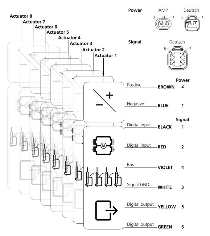
Please be aware that if the power supply is not properly connected, you might damage the actuator! The Green and Yellow wires from parallel connected actuators must NOT be interconnected
