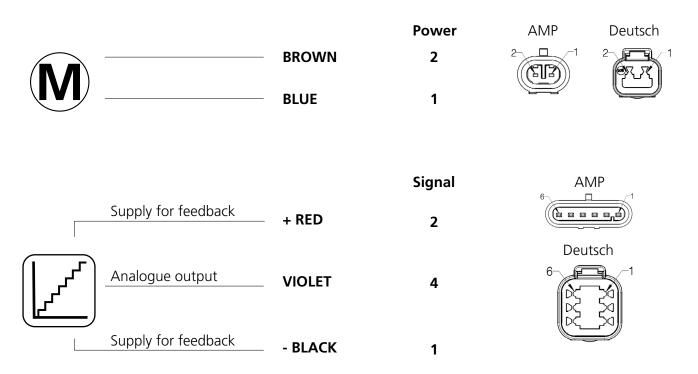
The signal power must be turned on at all times when the actuator is running, and minimum one second before it starts to run.
