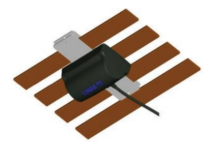
The massage motors are mounted on three slats with two brackets 0761010 and six M6 screws of good quality and two self-locking nuts. Four self-locking nuts inside the motor avoid that the mounting screws come loose.
