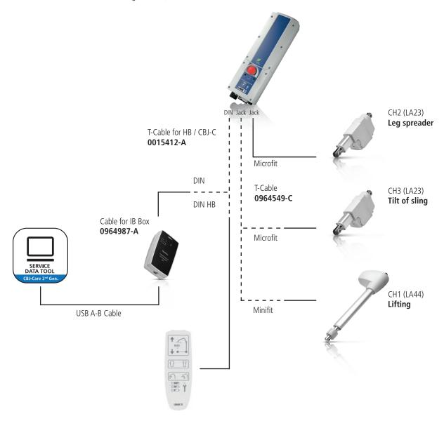
The T-Cable 0015412-A is needed if you do not have an activation button on the JUMBO Care control box.
