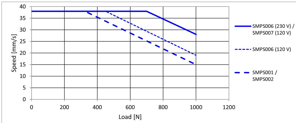
Figure 1 Two IC columns (equally loaded) with SMPS001/002/006/007
