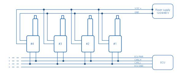
The power supply for the LINAK® CAN bus actuator should be kept separate from the CAN bus power supply, if such one exists.
