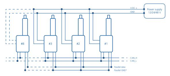
If there is a need for e.g. monitoring the real-time data of each actuator, it is possible to connect all actuators as nodes to the bus communication. This will provide comprehensive usage data, which can be used to enhance performance in the application. Similar to option 1, this requires that all actuators are connected to internal parallel communication.
