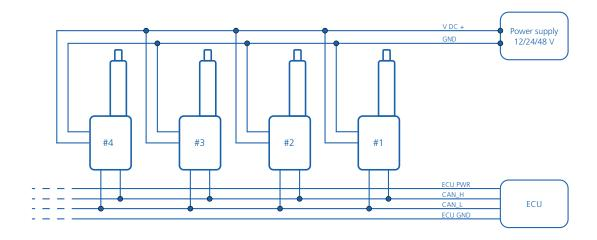
The power supply for the LINAK® CANopen actuator should be kept separate from the CANopen power supply, if such one exists.
