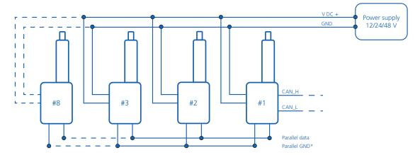
In a simple parallel setup there is only one actuator connected to the BUS communication. This actuator receives run commands and shares data with the BUS controller. The remaining actuators in the system are only connected to internal parallel communication. This way, the internal communication ensures that the system operates in parallel and stops in case of an obstacle, or when other errors occur on one of the actuators.
