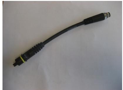
The connector pin layout has been chosen to enable use of standard DeviceNet M12 cables, passive TAPs (T-pieces) and terminators.
