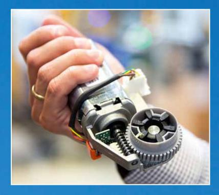
A motor-driven spindle rotates to move a tube with a nut forward and backward on the spindle. This generates a linear movement.
