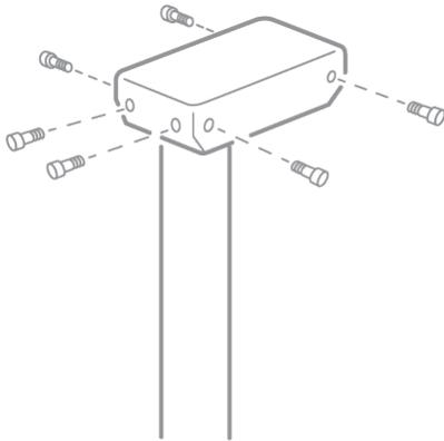
Use all 6 threaded mounting holes M6 for screws.
