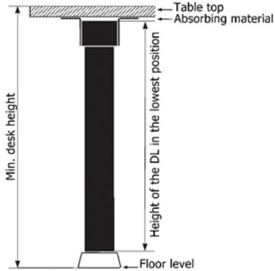
A suitable desk height in the lowest position can be obtained by mounting the lifting unit on a 6-8 mm bottom plate by means of 4 pcs. of M6 countersunk screws. We recommend you to use screws of min. quality 8.8. The thrust moment must not exceed 10 Nm in the bottom plate thread.
