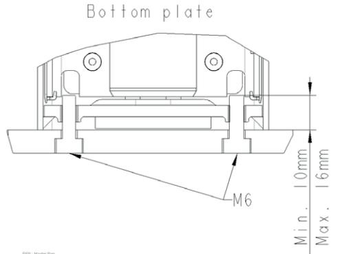
The 4 holes in the bottom of the column are placed from each other 58/34 mm respectively.
