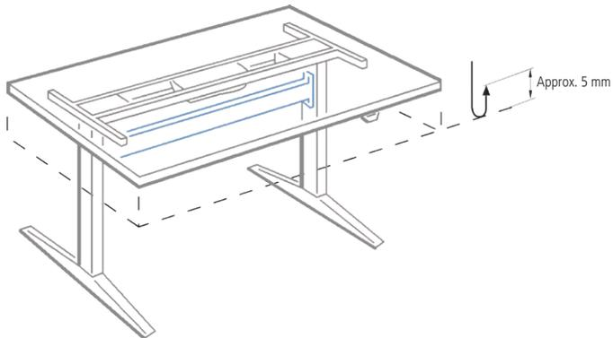
The CBD5 and CBD6 can control DL5 and DL6 in 2 parallel while the CBD4 can control DL5 and DL6 in 2, 3, and 4 parallel so that the desk is always kept horizontal.
