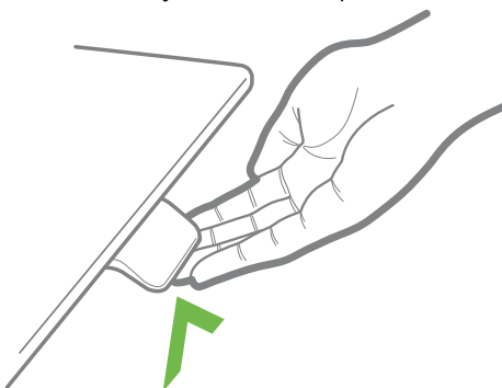
Figure 4 Tilt and hold the DPI to drive the desk up
