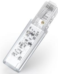
The Bluetooth® Adapter BLE2LIN002 allows you to adjust your LINAK product wirelessly from an app or a Bluetooth® hand control. Simply download the app, plug the Bluetooth® Adapter into your HOMELINE® control box, pair the adapter with your smartphone or tablet and your application can now be adjusted via your smartphone, tablet or HOMELINE wireless hand control.
