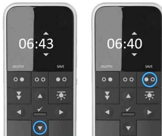
3. Use the 'left' and 'right' buttons to adjust the day of the week. Press the 'select' button or button 3 "SAVE" to save the day.
