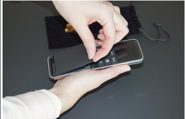
2. Put in the new batteries as indicated in the housing.
