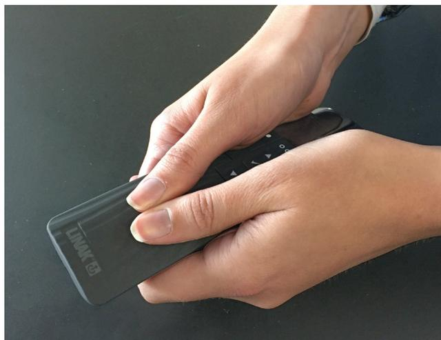
2. Put in the new batteries as indicated in the housing.
