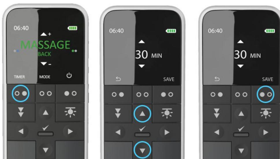
Note: If the timer in the HC40 is set to a higher number than what is configured in the actuator system as timer, the massage will stop according to the configuration in the actuator system.
