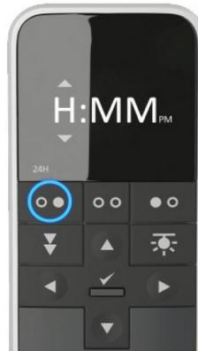
2. Adjust the time by using the 'up' and 'down' buttons on the keypad. Once the hours and minutes are adjusted, "SAVE" appears in the display. Press the 'select' button or button 3 "SAVE" to save the time.
