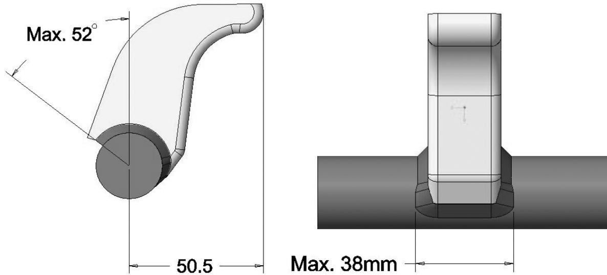
No bracket or welding outside this area 52° from vertical axis
