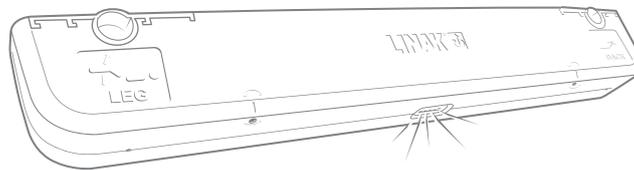
3. Press the two top buttons on the LINAK hand control at the same time.
