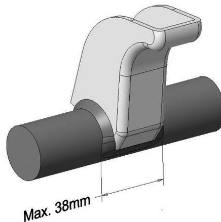
The dimension of the twist bracket including welding may not exceed 38 mm.
