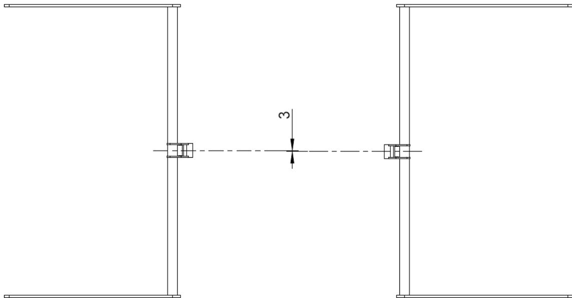
The shaft diameter must be  $\text{Ø}25.2 \text{ mm } +0.3 \text{ mm}/-0.2 \text{ mm}$
