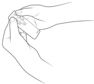
The Under Bed Light gives one long flash to indicate that the hand control and the TWINDRIVE are paired up. The TWINDRIVE stays in pairing mode and it is possible to connect more controls using the same procedure.
