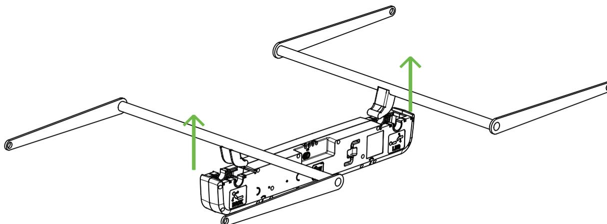
2. Slide each closing device on and press it into correct position.
