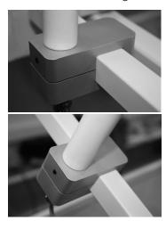
The FPP must be mounted in such a manner that it is secured against rotation. For this purpose the bracket end of the arm has 4 drilled holes - one of the 4 holes must be secured via the bracket with a slotted set screw with cone point (pointed screw). Otherwise it may slide away from the user when operated.
