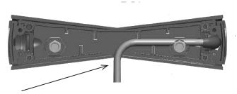
Location of the notch for the cable of the FS3 bed model.
