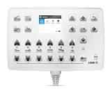
ACOD is an intelligent attendant control for hospital and nursing home beds, which is based on LINAK OpenBus<sup>™</sup> platform. It has up to 25 buttons, of which 7 are dedicated to display navigation, 13 LEDs and one 2.4" colour LCD display panel, allowing full functionality of the bed.
