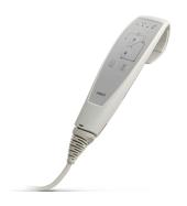
The HB30 hand control is designed for better user experience and ergonomic fit for the hands of caregivers. The compact size ensures one hand operation. The HB30 is especially suitable for patient lifts and other MEDLINE® and CARELINE® applications like couches, tables and chairs for treatment and examination. The HB30 is available in an analogue version and an OpenBus™ version.
