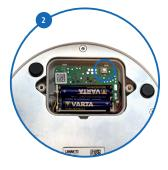
Activate Direct Pairing by pressing the button under the battery cover for 3 seconds. Buzzer and LED are now activated.
