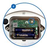
Confirm pairing by pressing the button under the battery cover. A double confirmation beep means that pairing is OK.
