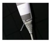
Step 1: Release the cable by pushing e.g. a screwdriver into the hole on the back of the hand control. Twist and release.
