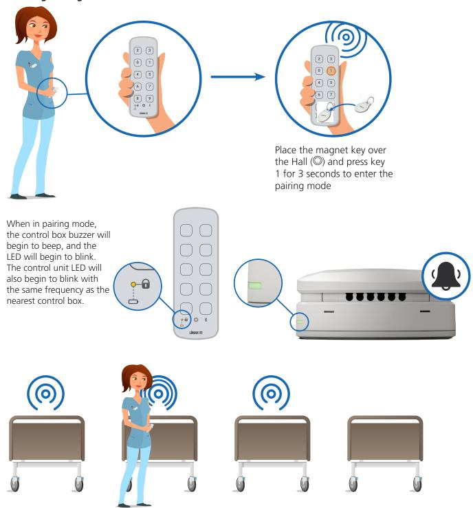
In pairing mode, the light/sound frequency will increase when the HB200 gets closer to a control box.
