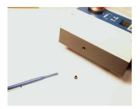
Only the end with the lowered notch must be used for adjustment of the potentiometer.
