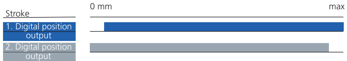
Figure 11 Endstop reached - Active low
