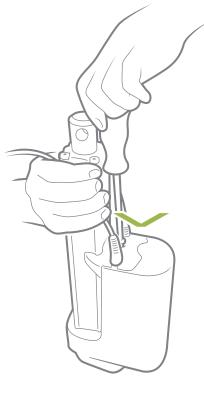
3. Slide the cover onto the actuator.
